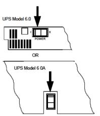
Power on the UPS Main Power Switch with the switch at the rear of the UPS.
