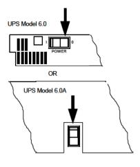
Power off the UPS Main Power Switch with the switch at the rear of the UPS.
